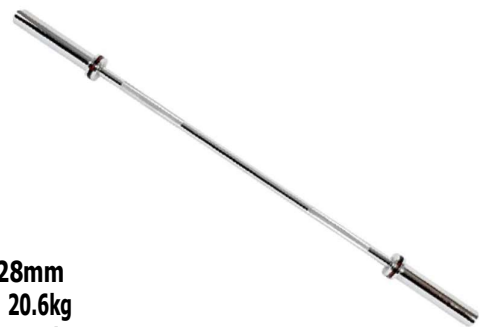
Olympic 7.2 FT chrome straight bar with solid end steel caps with Olympic training collars and 2 bronze bush and 4 needle bearing.
